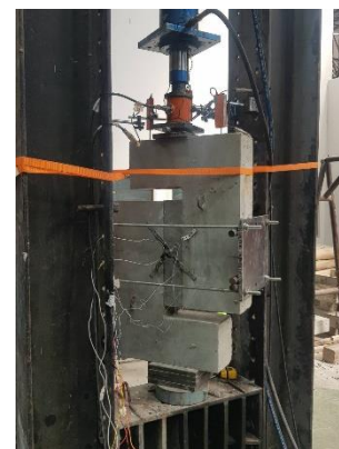
Figure 2. Push-off test setup configuration.
