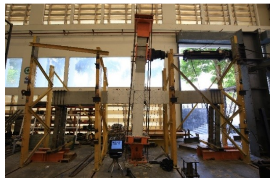
Figure 5. Failure of BC1S specimen at 6.00% drift ratio
