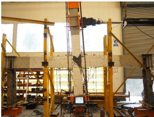
Figure 7 Failure of BC2J specimen at 6.00% drift ratio
