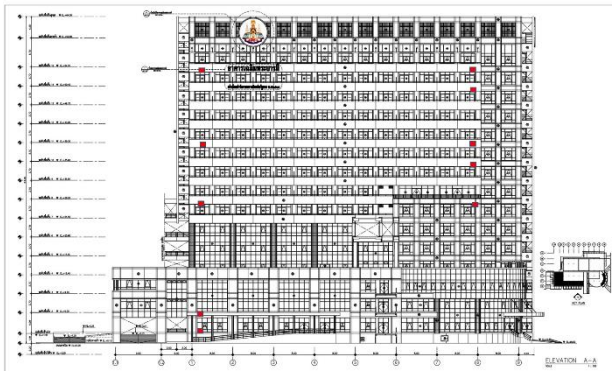
Figure 3. Location of installed low cost sensors
